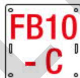
RFI 901 / 815 Sign for electric sections overhead CL-feeder. A2 type.
