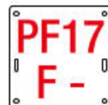
RFI 901 / 814 Sign for electric sections overhead CL-feeder. A1 type.
