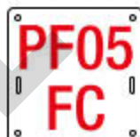
RFI 901 / 813 Sign for electric sections overhead CL-feeder. A type.
