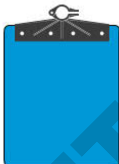
LIGHT BLUE PANTONE TYPE 299.C Coloration used in odd-numbered rail tracks (1 st directrix) with intermediate isolated overlap.
