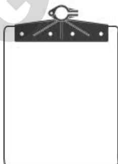
WHITE Coloration used for identification of railway portals, power suppliers and intermediate isolated overlap zones in whole line.
