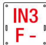
RFI 901 / 816 Sign for electric sections overhead CL-feeder. A3 type.
