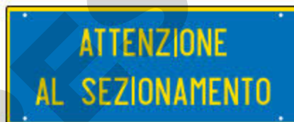
RFI 766 / 024 Warning sign for "ATTENTION TO ISOLATED OVERLAP".
